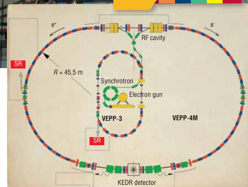
At the INP, VEPP-3/VEPP-4 are used in the acceleration storage complex for SR generation, VEPP-3 being a booster (intermediate) accelerator for the VEPP-4 collider (diagram on the right). Acceleration occurs in the range of energy from 360 MeV to 2 GeV; in the storage mode the accelerator can hold beams with an energy of 2 GeV and a current of about 100 mA for a long time (5–6 h). It is in this mode that the work using SR is conducted. Upper right: the rectilinear part of the VEPP-3 storage ring
