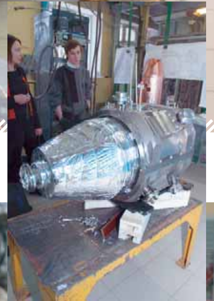
Superconducting solenoids operate at a very low temperature; therefore, each unit of a solenoid has a buffer volume of 200 liters for storage of liquid helium (its temperature is 4°K or — 269°C)
