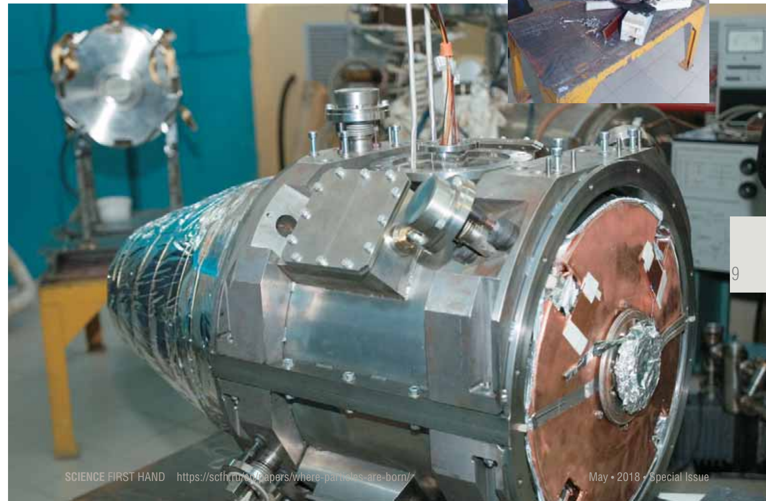
Superconducting solenoids operate at a very low temperature; therefore, each unit of a solenoid has a buffer volume of 200 liters for storage of liquid helium (its temperature is 4°K or — 269°C)
