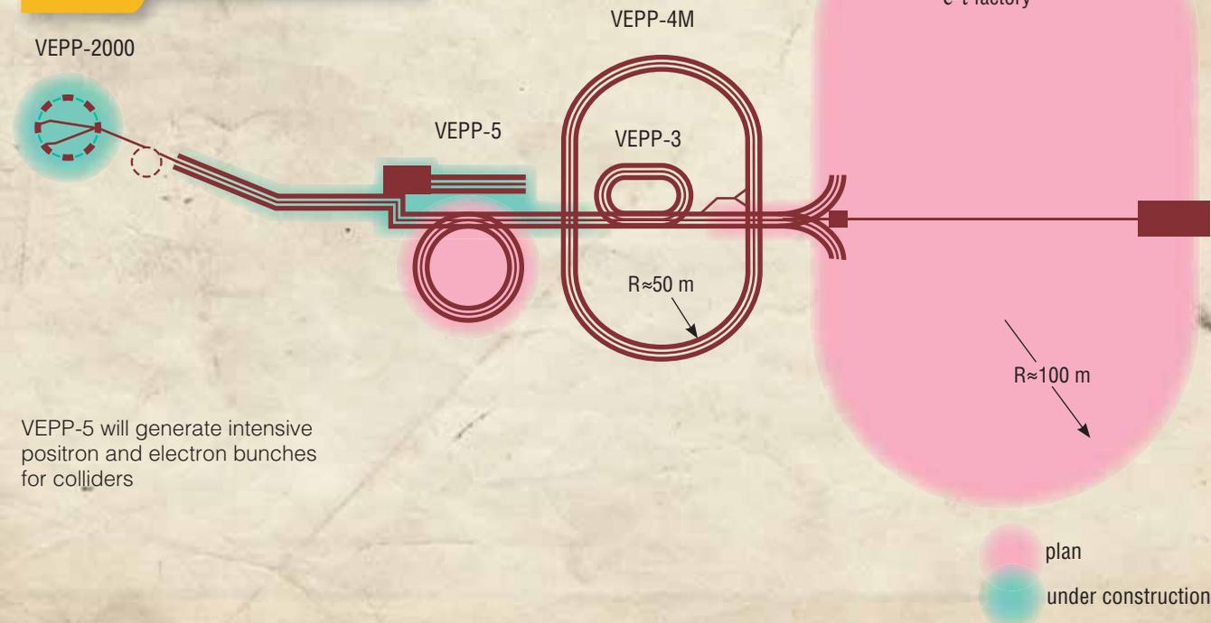
VEPP-5 will generate intensive positron and electron bunches for colliders
